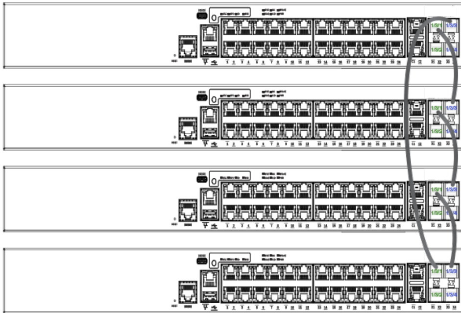
FIGURE 11 ICX 7150 24-port stack ring topology
