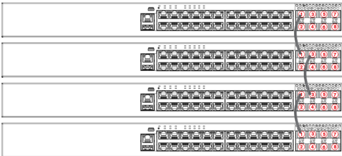
FIGURE 15 ICX 7250-24P linear stack
