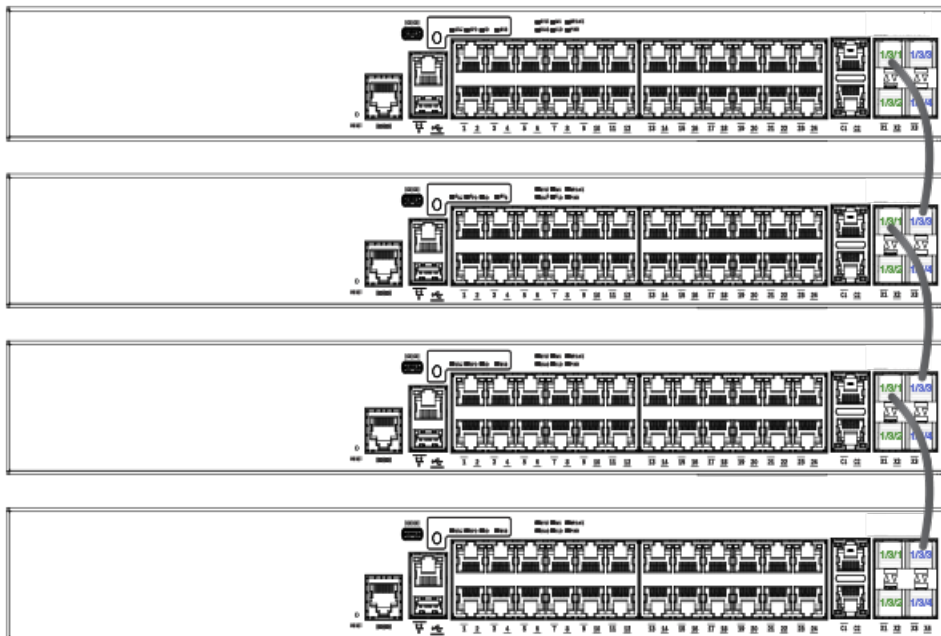
FIGURE 10 ICX 7150 24-port model, linear stack
